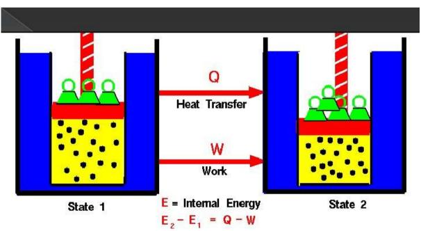
Any thermodynamic system in an equilibrium state possesses a state variable called the internal energy (E). Between any two equilibrium states, the change in internal energy is equal to the difference of the heat transfer into the system and work done by the system.
