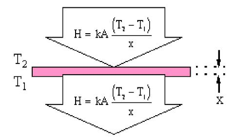
Assuming that the heat losses to the from sides of the sample are negligible, the steady state rate of heat transfer (H) by conduction
