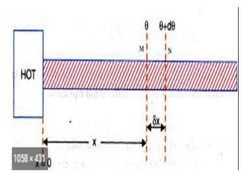
Let us consider a long metal bar of uniform cross –sectional area A, heatedat one end .The bar lies along the x – axis whose origin is at the hot end . Heat flowsalong this axis .Now consider a thin slice with two parallel planes A and B perpendicular to the length of the bar at distances x and x + $\Box x$  from the hot end . If  $\theta$  be the temperature of the plane  $\mathrm{Aand} d\theta/dx$  be the heat which leaves the slice at B per second .Then
