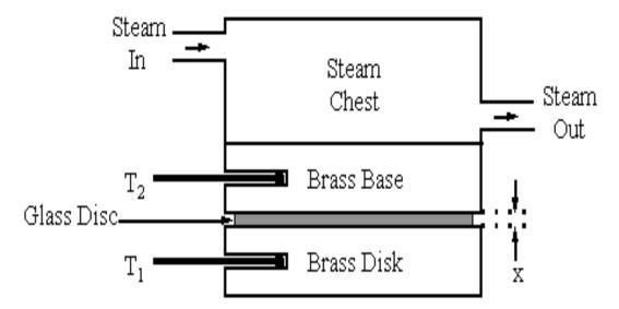
Similarly the temperature of the brass disk (measured by  $T_1$ ) is very close to the temperature of the lower glass surface. In this way the temperature difference across such a thin sample can be accurately measured.
