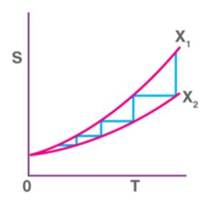
From the graph, it can be observed that – the lower the temperature associated with the substance, the greater the number of steps required to cool the substance further. As the temperature approaches zero kelvin, the number of steps required to cool the substance further approaches infinity.
