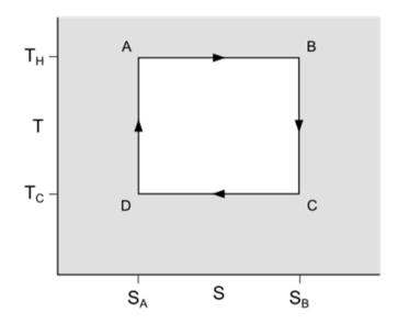
A Carnot cycle acting as a heat engine, illustrated on a temperature–entropy diagram. The cycle takes place between a hot reservoir at temperature TH and a cold reservoir at temperature TC. The vertical axis is temperature, the horizontal axis is entropy.
