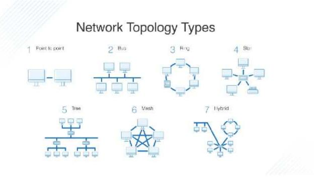
There are also hybrid networks such as a star-bus hybrid, star-ring network, and mesh networks with connections between various computers on the network. Mesh networks ideally allow each computer to have a direct connection to each of the other computers.
