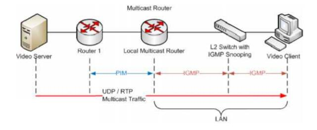
IGMP operates between a host and a local multicast router. Switches featuring IGMP snooping derive useful information by observing these IGMP transactions. Protocol Independent Multicast (PIM) is then used between the local and remote multicast routers, to direct multicast traffic from hosts sending multicasts to hosts that have registered through IGMP to receive them.
