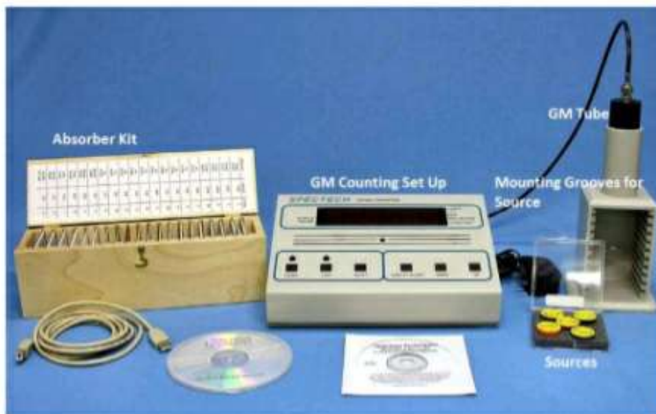
Figure 1: Experimental set up for GM Counter based experiments. Taken from the company manual http://www.spectrumtechniques.com/resources/instrument-manuals/
