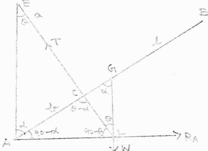
(ii) its weight  $w$  acting vertically downwards through  $G_r$ , the mid point of  $AB$  and. (6)
