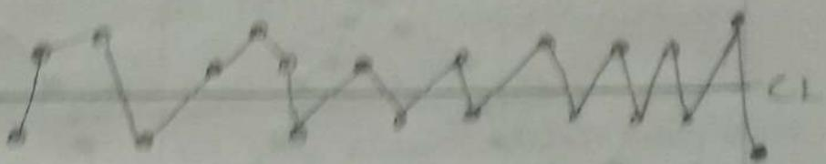
5. Presence of Trends. The Trends exhibited by sample points on the control chart are also an indication of assignable cause. Trend pattern, a phenomenon usually observed in engineering industry, indicates the gradual shift in the process level.
