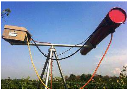
Figure. A propane-fired canon.
