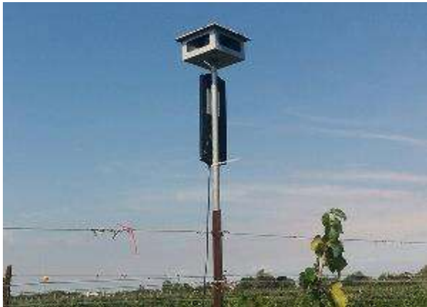
Figure. An electronic sound device (squawker)
