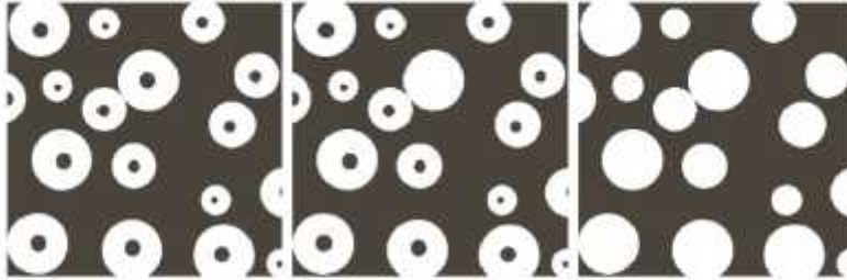
FIGURE 9.16 (a) Binary image (the white dot inside one of the regions is the starting point for the hole-filling algorithm). (b) Result of filling that region. (c) Result of filling all holes.
