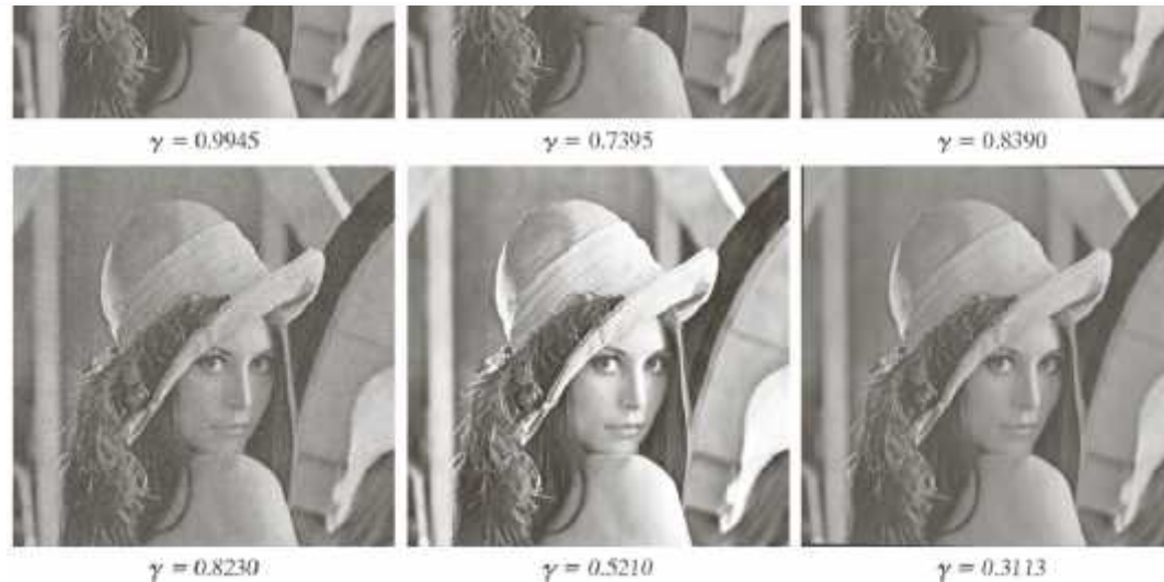
FIGURE 8.54 Attacks on the watermarked image in Fig. 8.53(a): (a) lossy JPEG compression and decompression with an rms error of 7 intensity levels; (b) lossy JPEG compression and decompression with an rms error of 10 intensity levels (note the blocking artifact); (c) smoothing by spatial filtering; (d) the addition of Gaussian noise; (e) histogram equalization; and (f) rotation. Each image is a modified version of the watermarked image in Fig. 8.53(a). After modification, they retain their watermarks to varying degrees, as indicated by the correlation coefficients below each image.
